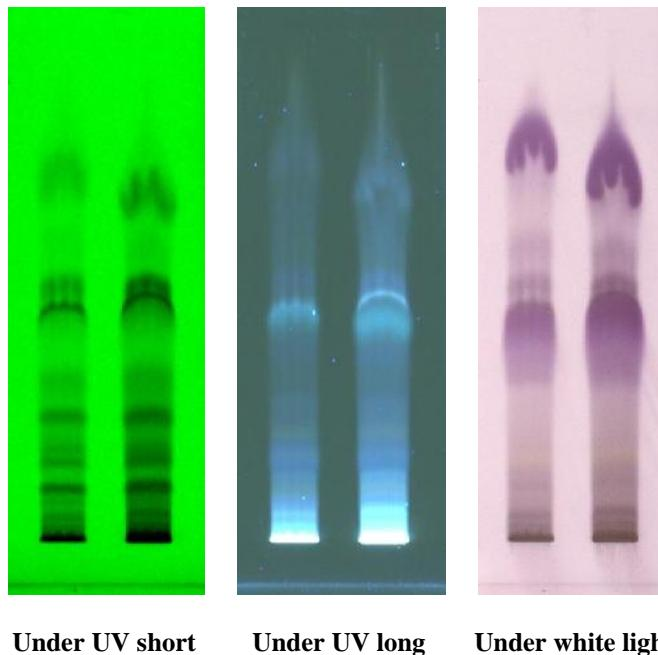
**Fig (2b): TLC photodocumentation of Chloroform extract of Murukkanvitai mathirai Viewed in UV short;Viewed in UV long; After derivatisation using vanillin-sulphuric acid viewed in visible light Solvent system – Toluene; Ethyl acetate: Formic acid (5:1:2 drops)**
