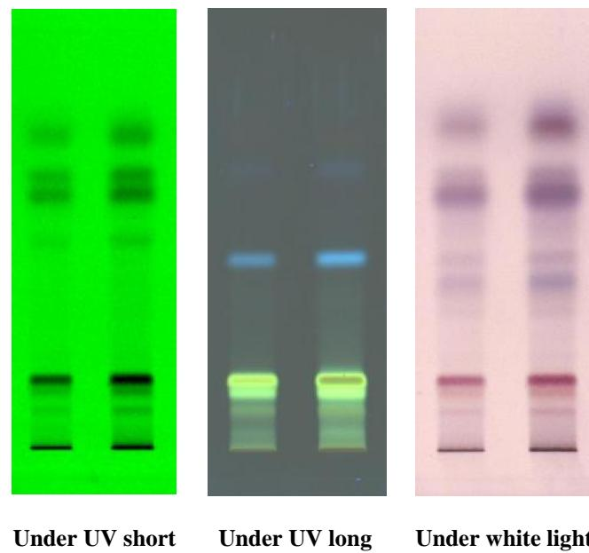
**Fig (1d): HPTLC profile of Chloroform extract of *Curcuma aromatica* Salisb. (Kasthuri Manjal), Rhizome; Viewed in UV short; Viewed in UV long; After derivatisation using vanillin-sulphuric acid viewed in visible light; Solvent system – Toluene: Ethyl acetate (5:1)**
